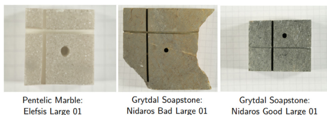
Fig. 10. Some of the stone slabs used in PRESIOUS accelerated erosion experiments [16]. The stones named Elefsis consist of pentelic marble, while stones names Nidaros consist of grytdal soapstone, representing the material of two monuments that were considered in the PRESIOUS project, the Demeter Sanctuary in Elefsis (Greece) and the Nidaros Cathedral in Trondheim (Norway) respectively.
