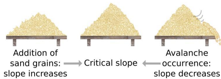
Figure 4: This figure depicts Bak et al.'s sand pile metaphor, which is a SOC model. The addition of grains creates at some point a minimally stable point, the addition of more grains makes the model stabilize back to this minimally stable point (23). [“The sand pile model”, from Self-organized criticality as a fundamental property of neural systems, by Hesse et al. (2014). URL: https://www.researchgate.net/figure/The-sandpile-model-The-classical-thought-experiment-motivating-self-organized_fig2_266626997 , Figure license ( CC BY 4.0), full terms: Creative Commons Attribution 4.0 International
