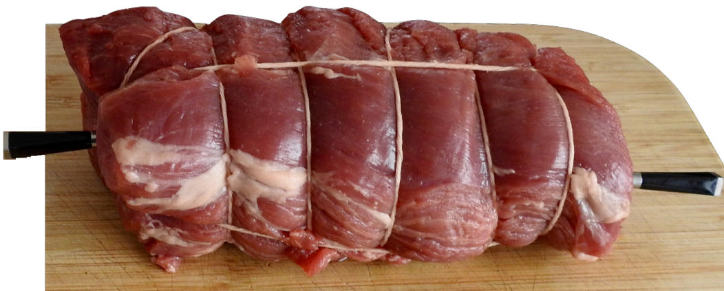
Figure 8.4: The tenderloin sample. With two thermal sensors insert.
