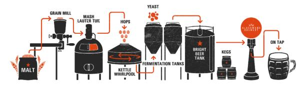
**Figure 2.4:** Illustration of the main processes in beer brewing: malt milling, mashing, lautering, boiling, whirlpool, fermentation, filtration and dispensing (27). Figure from (27).
