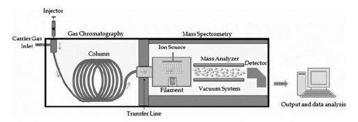
Figure 2.6: Schematic overview of the main components of gas chromatograph-mass spectrometer instruments. Adapted from (33).
