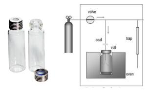
Figure 2.5: Empty glass vials with screw tops (left) and schematic diagram of the HS trap system (right). In the schematic diagram, it can be seen that the equilibrated vial is being pressurized with carrier gas. The pressurized gas will be released from the vial into the adsorbent trap, where the volatile compounds are collected before being thermally desorbed and introduced into the GC column (7). Figure adapted from (7, 31).
