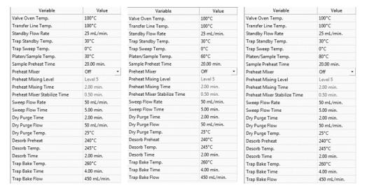
**Figure C.1:** The three methods used for the headspace sampling. All parameters remained the same except from the platen/sample temp., which was set to 30 °C, 60° C and 80 °C, respectively.
