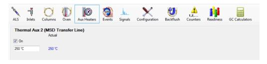
Figure C.5: GC Aux heater parameters
