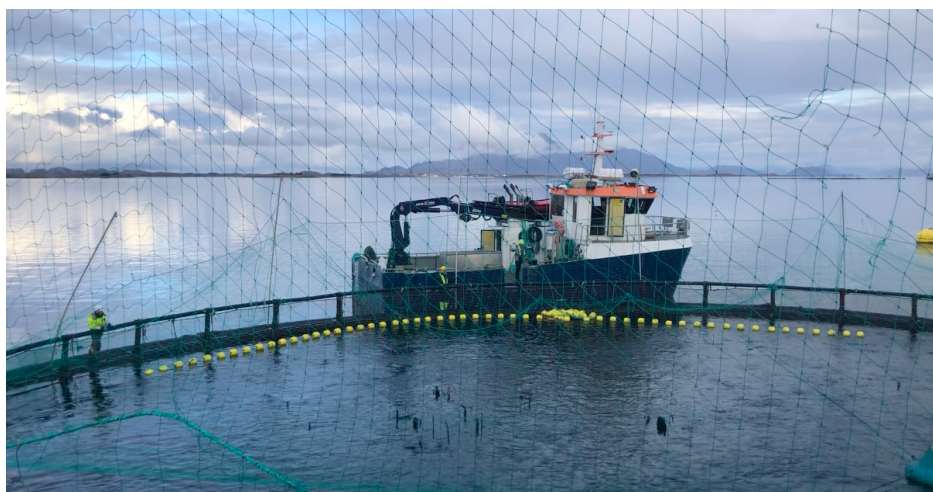
Figure 2.5: Crane on service vessel places the swipe net in the water.
