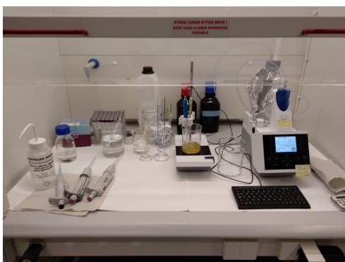
Figure 2.4: Titration equipment set up with PV analysis of one sample in progress
