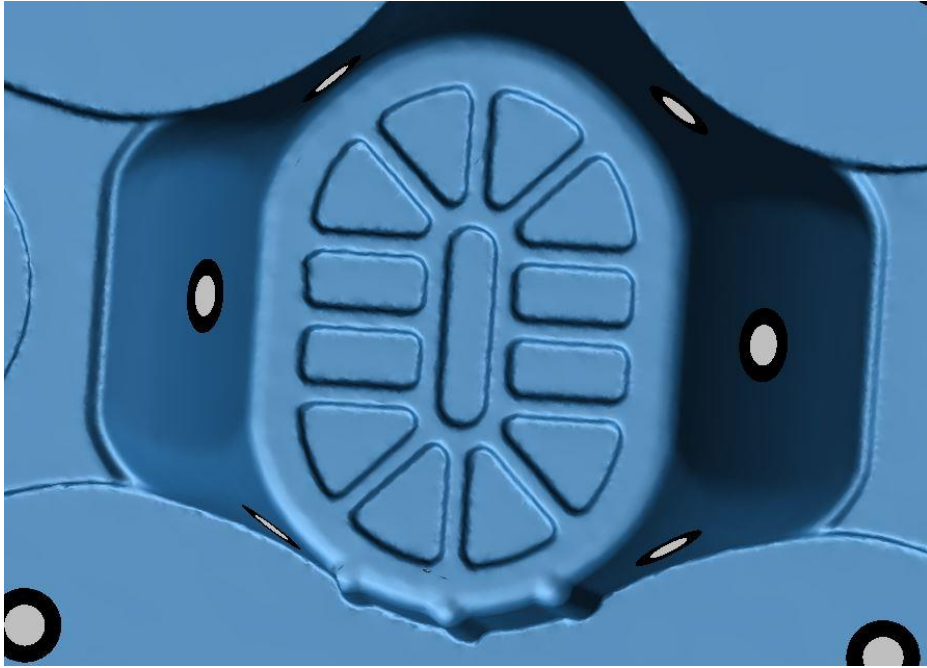
Figure 67: Closeup of the details on the filter cover of the cavity 3D-scan
