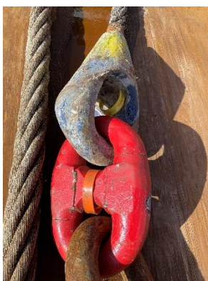
Figure 31 – Kenter shackle connected to socket (Author's photo).
