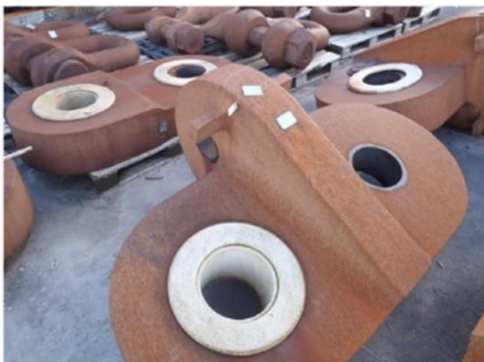
Figure 35 – Coupling plate (Lie, 2021).
