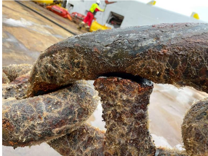
Figure 22 – Loose stud in chain (Author’s photo).
