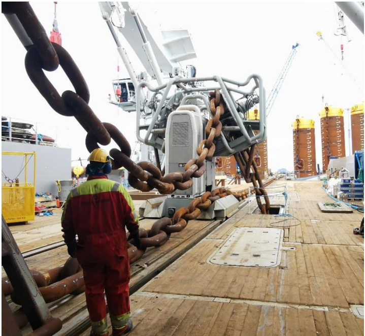
Figure 63 – Island Victory chain hauler (Island Offshore, 2020).
