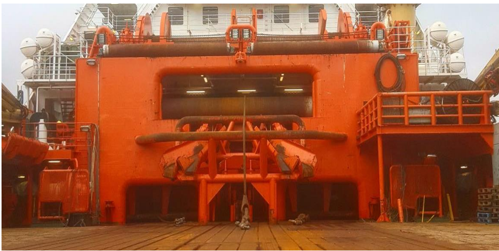
Figure 59 – N. Prosper fixed chain chutes (Author's photo).
