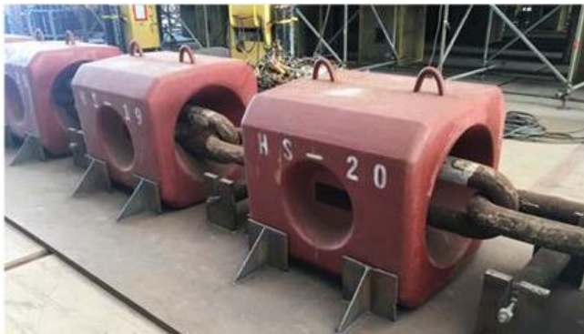
Figure 15 – Single shell cast clump weights added to chain (Kai-Tung et al., 2019).
