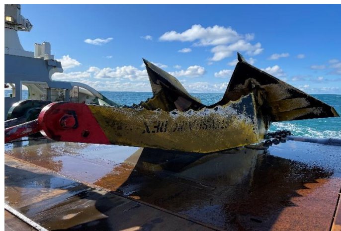
Figure 64 – DEA resting on back for launching (Author's photo)
