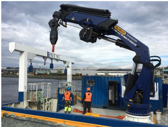
Figure 1.2: Palfinger crane PK-65002-M mounted in the NTNU Gunnerus ship
