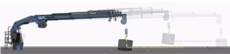
Figure 5.14: Kinematic Simulation of the maritime crane using NX Motion
