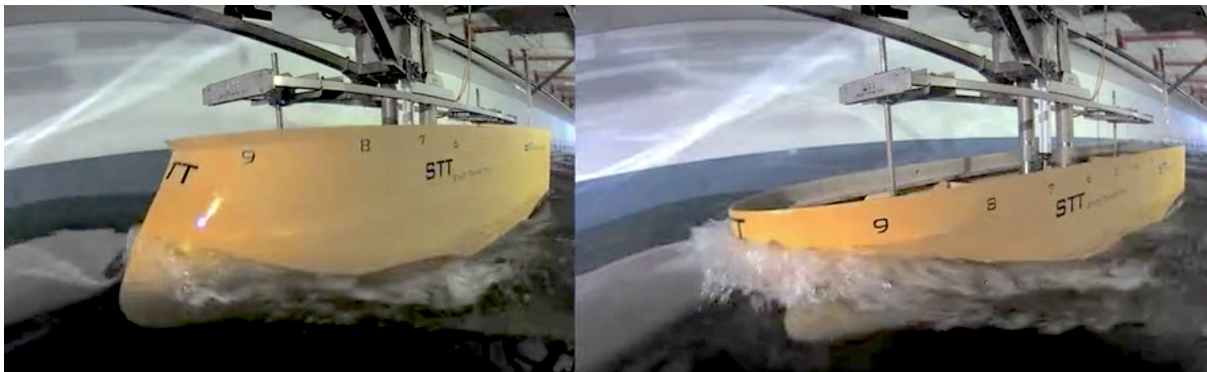
Figure 2.2: Model Test Comparison X-Bow vs Conventional Bow [5]
