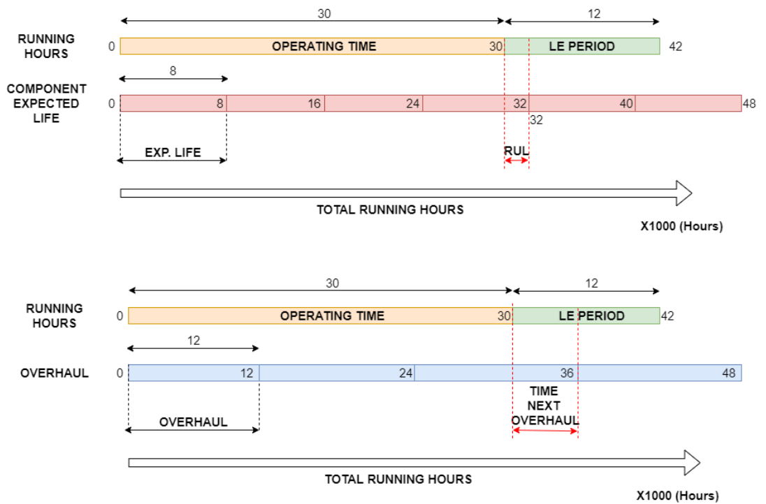
Figure 2. Predicting RUL and Next Overhauling for a Component of a Diesel Engine .
