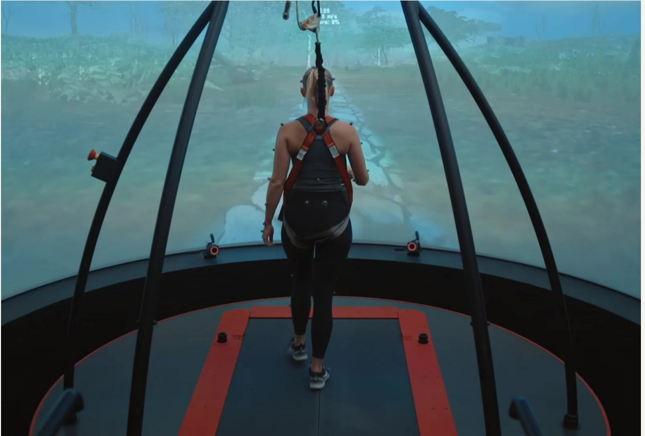
Picture of CAREN (Computer Assisted Rehabilitation Environment) in use. The system is one of the more advanced ways to use VR or games for rehabilitation.
