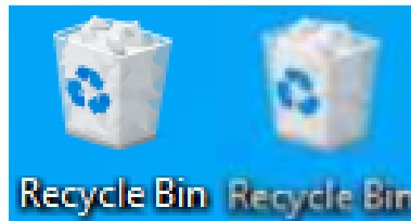
Figure 20: Zoomed in view of recycle bin uncompressed and compressed at 40 quality
