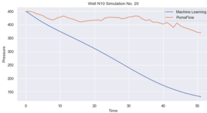
Figure 5.13: Experiment 5: This figure compares the ML-based simulations and PumaFlow TM physics-based simulations at a sample well (N10) for simulation No. 20 (test case).
