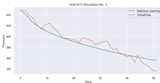
Figure 5.11: Experiment 4: This figure compares the ML-based simulations and PumaFlow TM physics-based simulations at a sample well (N10) for simulation No. 2 (training case).
