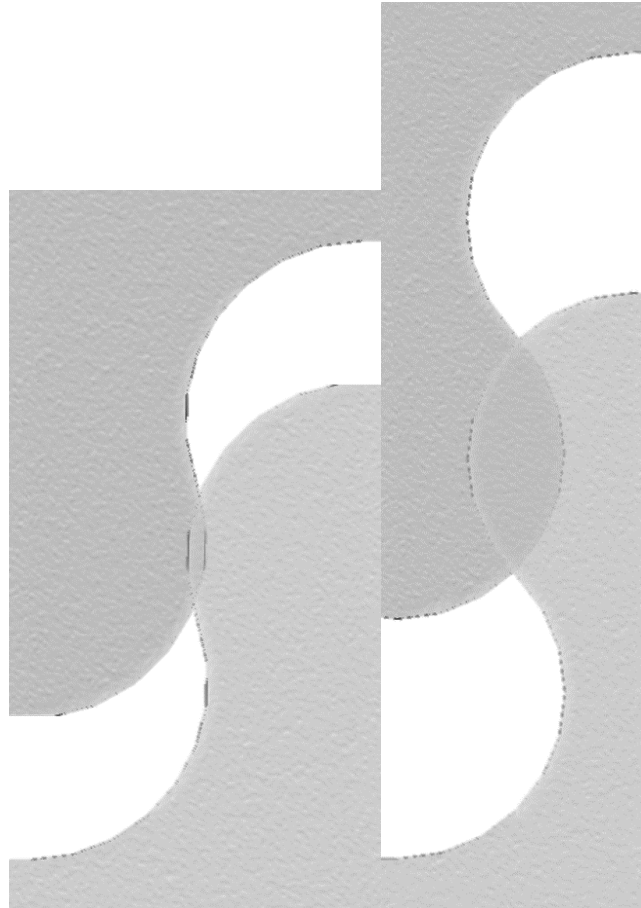
Figure 8: A 20-degree suture must deform less to pull out the male part from the female part than a 40-degree suture.
