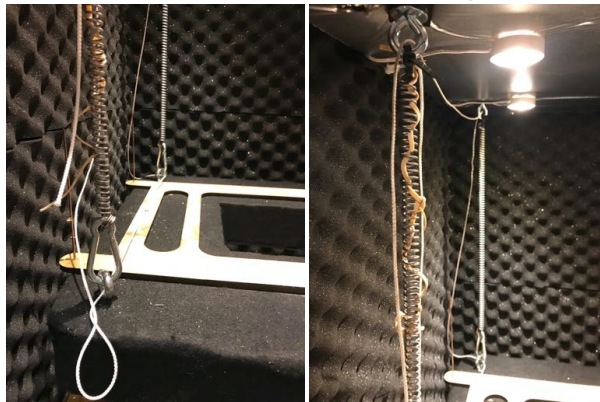
(b) The anti vibration chamber with closeup on the springs
