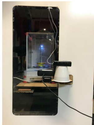
Figure 4.8: Experimental setup where the insulin pump is leveled at the same height as the top of the liquid
