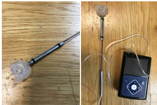
(a) The tube attached to thin wire with duct tape and thread
