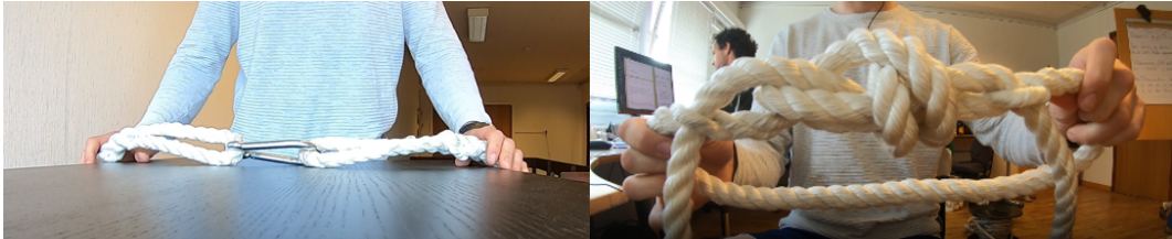
Figure 46: Splicing by carabine and eye splice (left) and knot (right).
