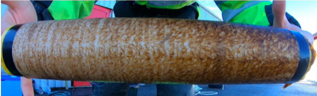
Figure 14: Seeding line spun tightly around a PVC-pipe (Seeding spool)
