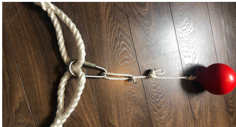
Figure 49: Splicing of two kelp lines and a buoy
