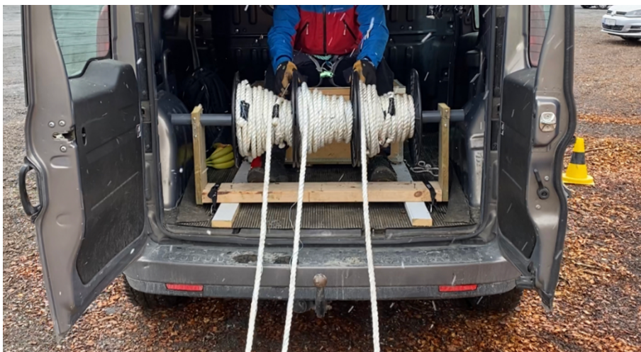
Figure 53: Deployment test using 3 drums from a car.
