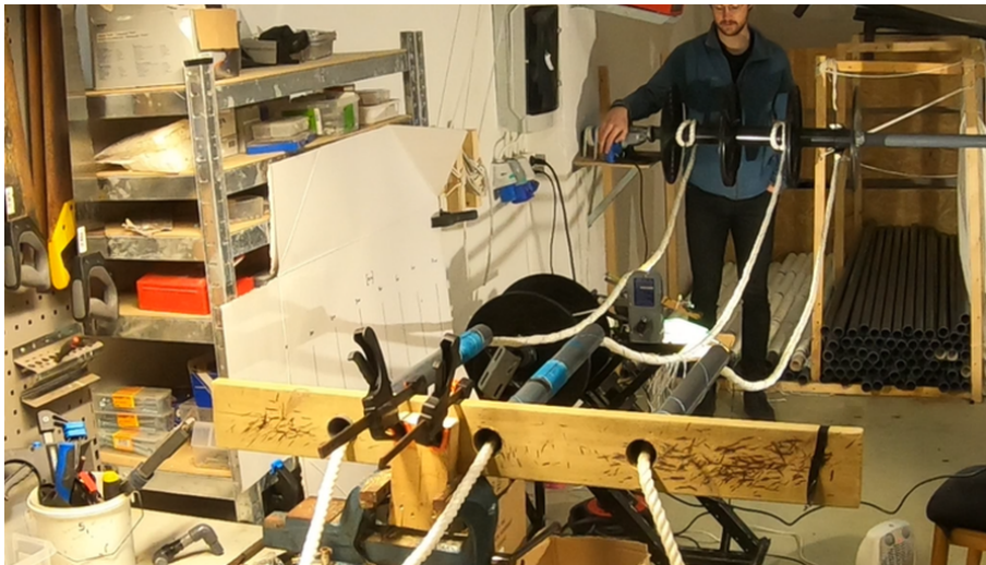
Figure 52: Combining test at the workshop using 3 drums
