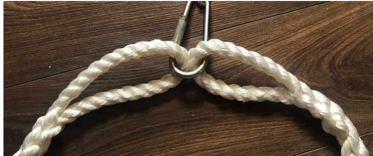
Figure 48: Splicing of kelp lines using a carabiner hook
