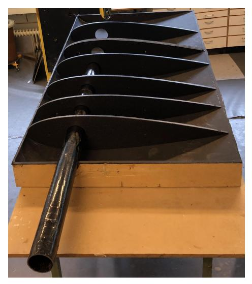
Figure 51: Mainsail with ribs and mast placed in the mainsail mould.
