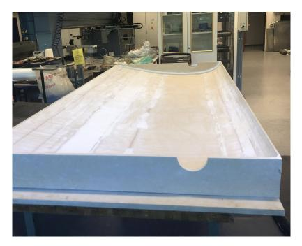
Figure 27: Mainsail Mould after assembly of milled components and filler applied.
