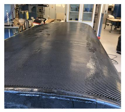
Figure 53: Mainsail shell after demoulding.
