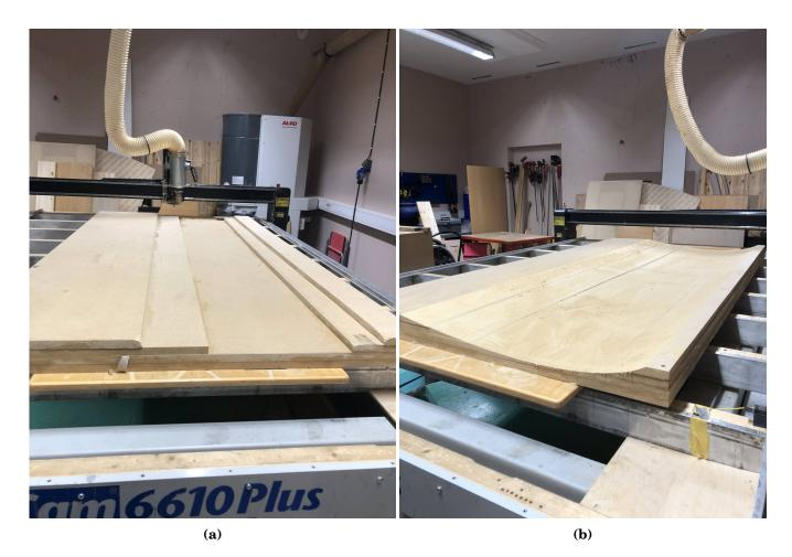
Figure 26: (a) Lower part of mainsail mould ready for milling, (b) Lower part of mainsail mould after milling.
