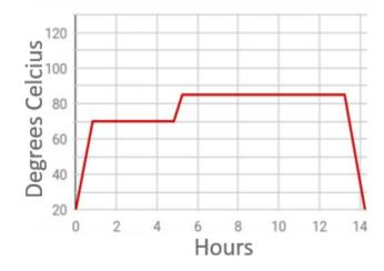
Figure 33: Low oven curing cycle was chosen for the ribs [I.7].
