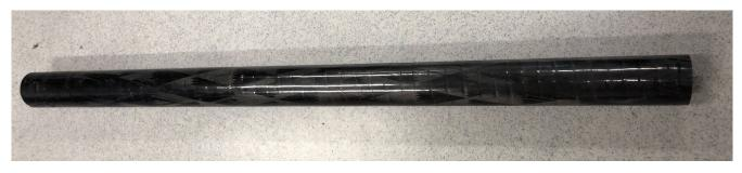
Figure 54: The CFRP mast with ends cutted.
