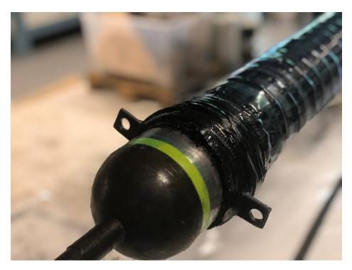
Figure 37: Illustration of the profiles attached to ease demoulding.
