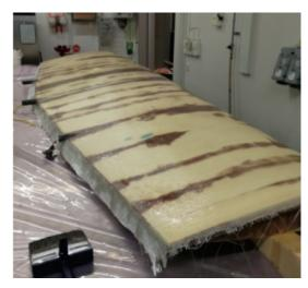
**Figure 1:** Wingsail produced as a sandwich structure with foam core [3].
