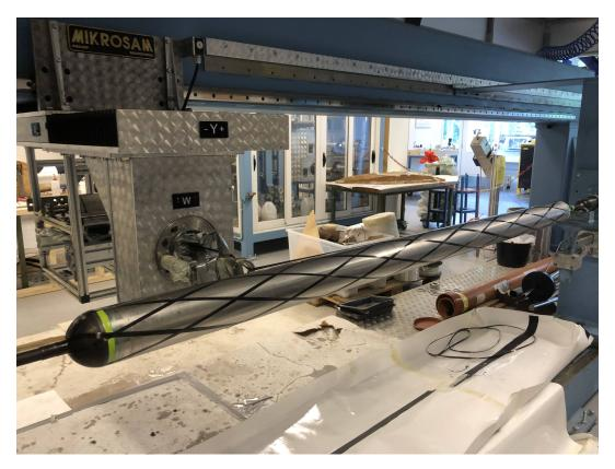
Figure 35: Start of the first layer of PAN carbon fiber wound onto the mandrel.
