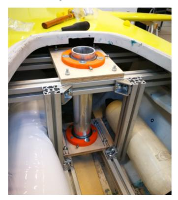
**Figure 61:** Suggestion for a ball bearing mast foot which was used in a similar project at the university KTH in Sweden [3].
