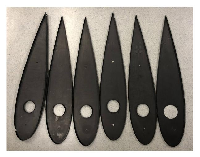
Figure 56: All six ribs trimmed and demoulded.
