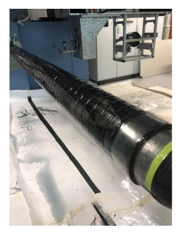
Figure 36: After the filament winding process was done with ends cut away and vacuum-bag strips attached.
