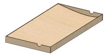
Figure 24: Milled mainsail mould components assembled together.
