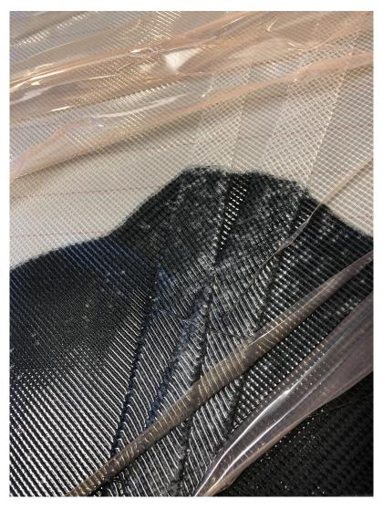
Figure 52: From the Mainsail production, air bubbles was observed in the infusion process.
