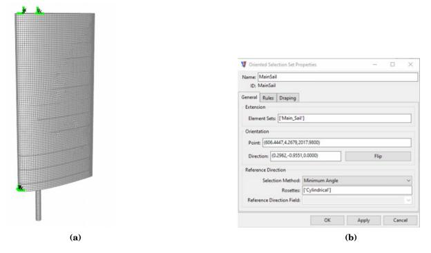
Figure 85: (a) Rosette definition, (b) Oriented Selection Set Properties.
