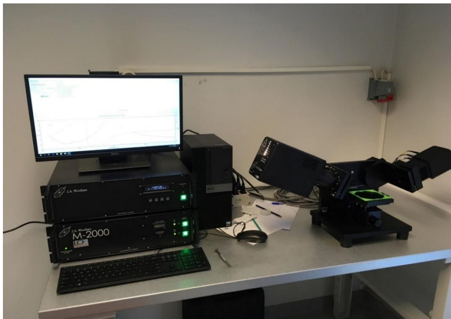
Figure 3.4: Setup for the ellipsometry to characterize the samples
