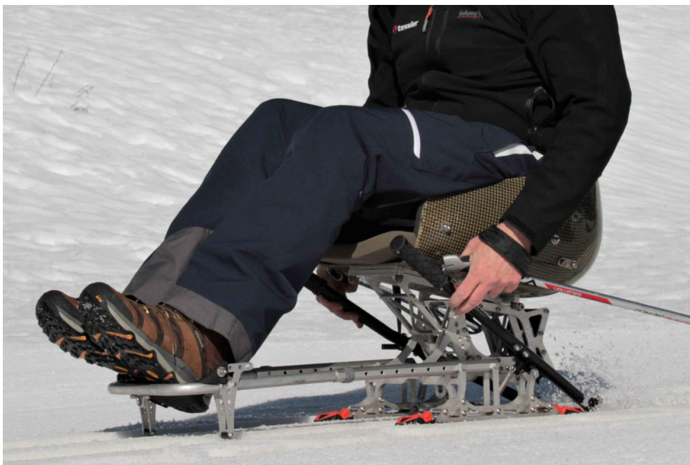
Figure 1.1: An adjustable CCSS with brakes, Tessier's Eskaip. [2]
