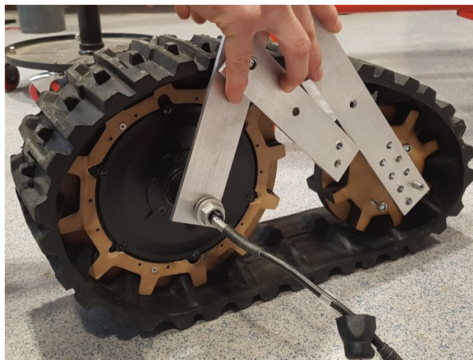
Figure 5.8: Assembling the drive system of the first track prototype — a set-based prototype with adjustable length of suspension bars in aluminum.
