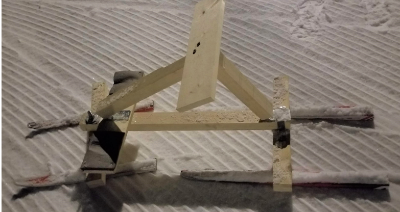
Figure 4.4: Prototype exploring turning. Vertical bolt acting as pivot point to enable rotation of frontal ski pair. A spring is connected to make forward the preferred direction.
