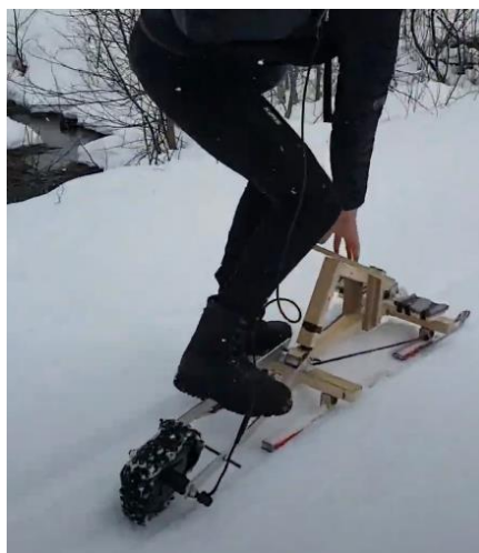
Figure 4: Testing of varying normal force on the drive wheel.
