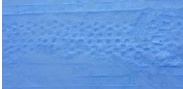
Figure 6: The mark outside the ski track from the ski and the studded tire, implying no slip and low indentation depth.
