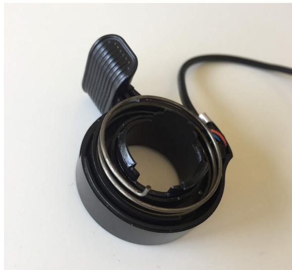
Figure 7.11: Thumb throttle with spring.
