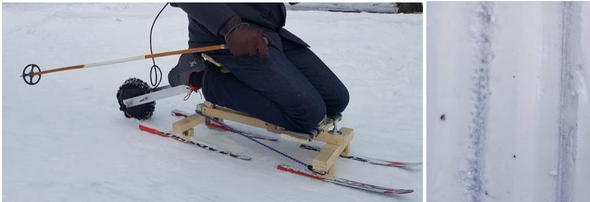
Figure 2: First test of small wheel and mark left in the ski track.
