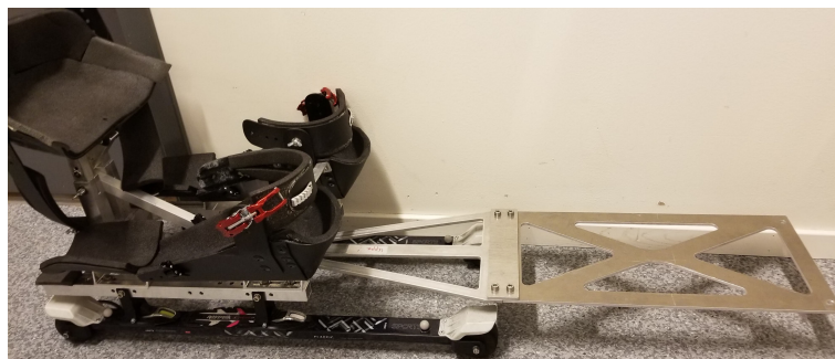
Figure 3.1: The CCSS with Rollerskis used on the big treadmill. The plate in front was connected to an aluminum track for safety.
