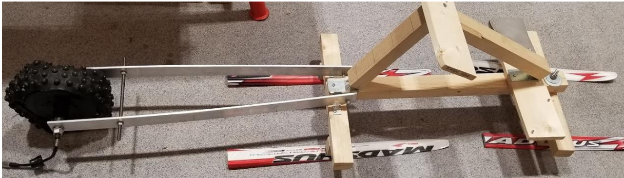
Figure 3: Test setup based on previous Turning prototype.
