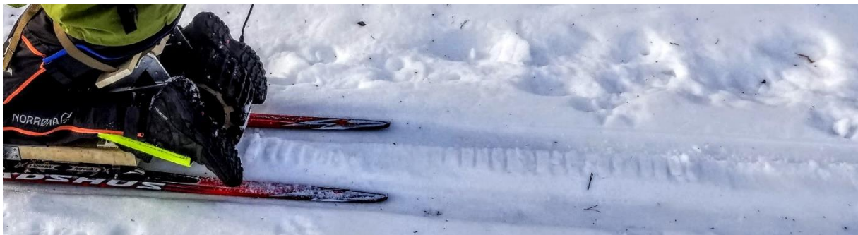
Figure 11: The prototype with rubber tracks and its impression on the middle of the ski track.
