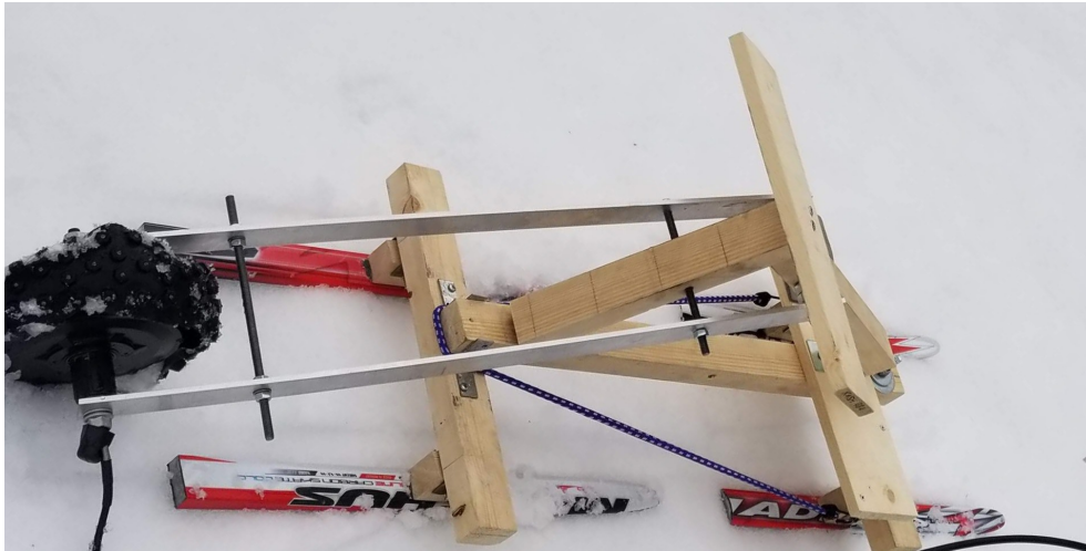
Figure 6.2: An initial prototype with an H-shaped bottom frame.
