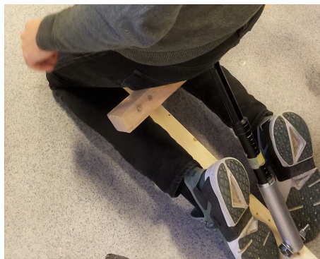
Figure 3.9: First physical representation of the Damper Model with a seat post.
