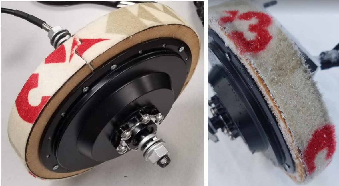
Figure 5: The state of the skins before and after testing.
