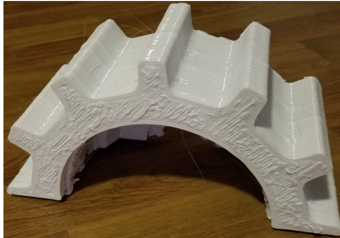
Figure 5.10: Half of the drive wheel sprocket printed to fit outside the hub motor with printing layer direction to resist shear stress from acting forces.
