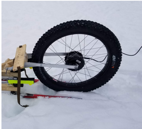
Figure 5.4: The commercial fatbike wheel connected to the chassis.
