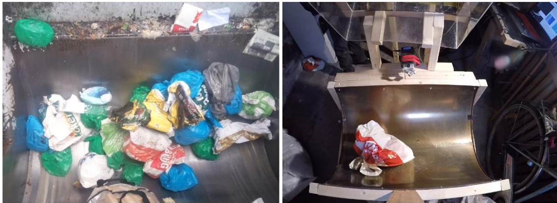
Figure 2: The landing tray of a waste collection truck under operation is shown on the left and the test rig on the right.
