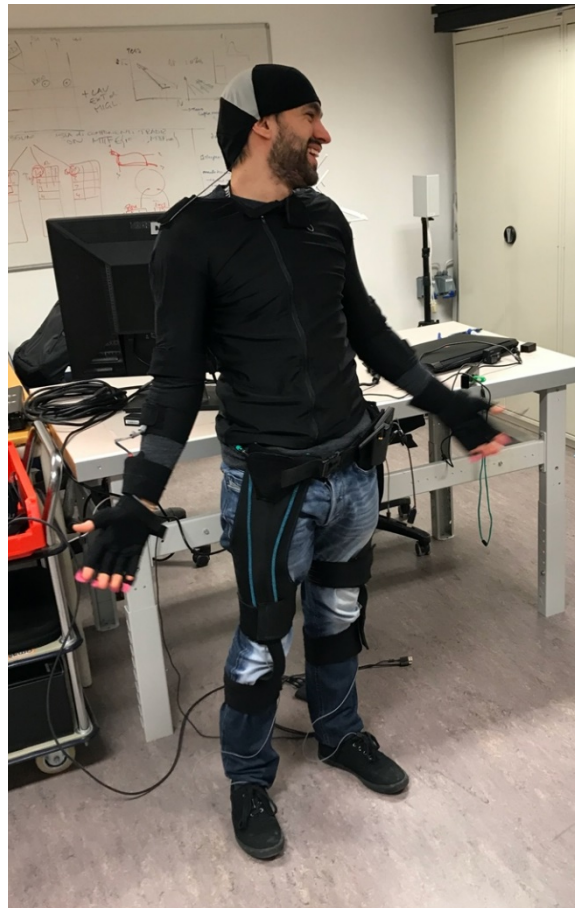
Figure 4.5 Test operator wearing an inertial motion capture suit in the Logistics 4.0 Laboratory at NTNU
