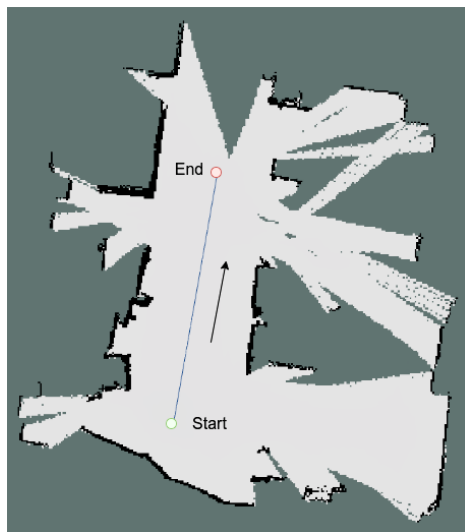
Figure 7.3.: The trajectory followed by the KMR down the hallway, based on wheel encoders, referred to as the ground truth. The map is created by RTAB-Map.
