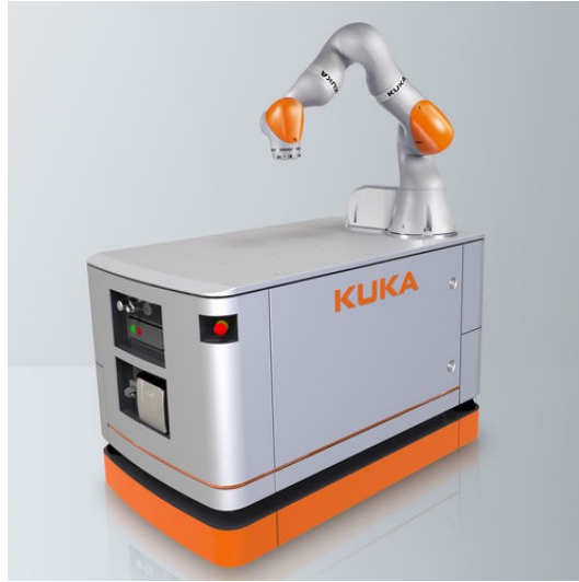
Figure 3.1.: KMR iiwa is composed of a mobile platform and a lightweight manipulator [24].
