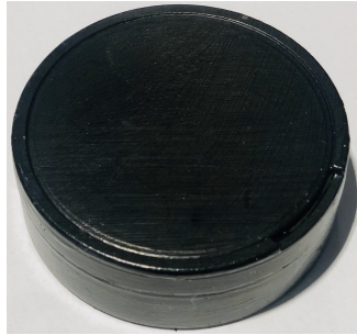
Figure 5.7.: The black circular box used for object detection and grasping throughout the project. The box has a diameter of 7 cm.
