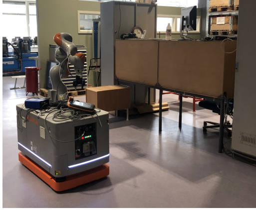
Figure 8.4.: Experimental area for testing the voxel layers with obstacles only detectable by the cameras.
