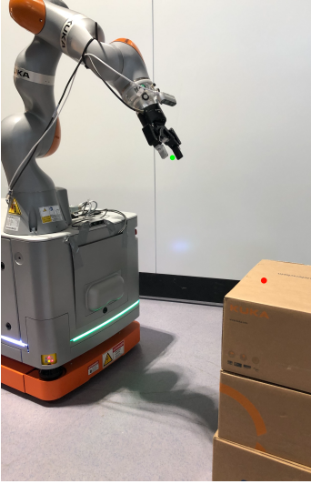
(a) The robot is placed in front of stacked cardboard boxes. The gripper middle point and the goal pose is denoted by the green and red markers, respectively.
