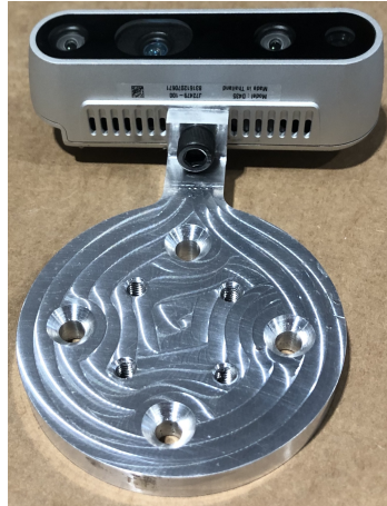
Figure 5.2.: The adapter used to connect the gripper to the media flange of the LBR.
