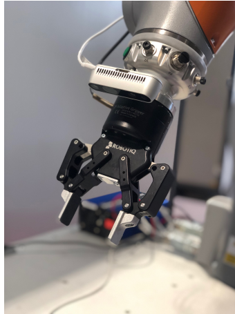
Figure 5.3.: A D435 camera is mounted at the end-effector.
