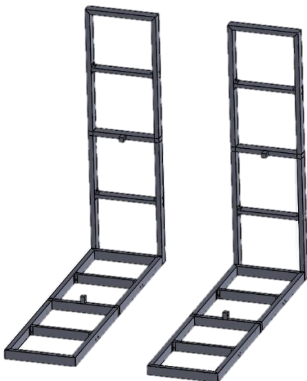
Figure 4.5: Four frames put together to form a flood wall. The middle is empty, but can be replaced with a solution that can make this flood wall flexible.
