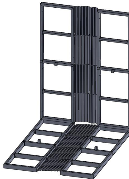
Figure 4.14: FFC2 expanded, notice that the hinges are not connected in the corner
