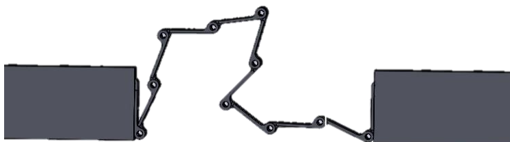
Figure 4.23: Illustrates the problem when the hinges can rotate freely. They can not be expected to stack nicely by them self
