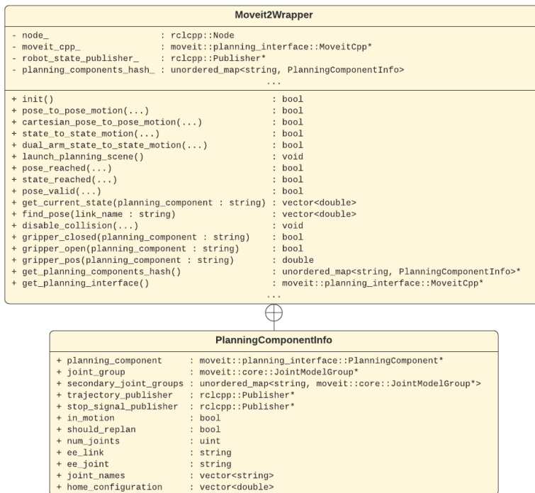
Figure 6.17: Simplified UML diagram of the Moveit2Wrapper class.
