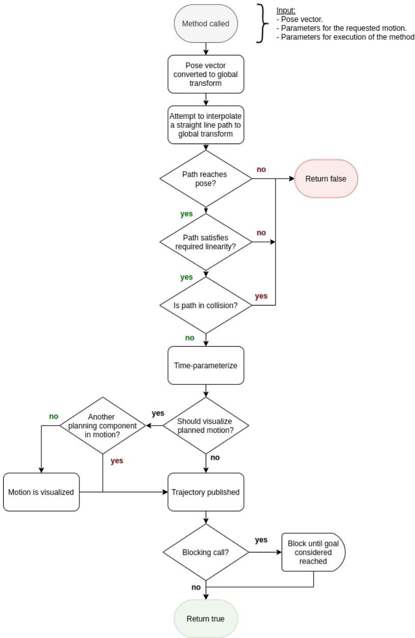
Figure 6.19: Flow chart of the execution flow of a linear Cartesian motion method.
