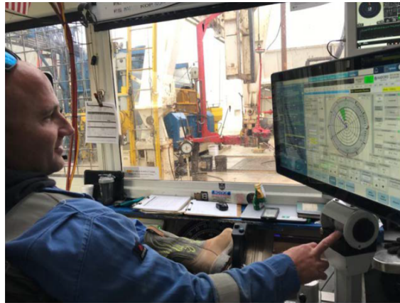
Figure 3.15: Driller using digital RAP (from Isbell et al. 2021)
