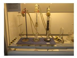
Figure 5.6: Core cleaning by Soxhlet extraction.
