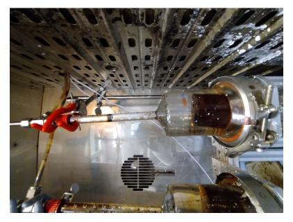
Figure 6.23: Observation of oil droplet spread on the surface of core sample B1.
