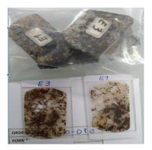
(a) Thin section images of C1 and C3 and their corresponding end-caps E1 and E3 respectively.
