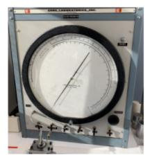
Figure 5.7: Helium Porosimeter.
