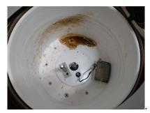
(b) Salt and oil droplets seen in the centrifuge machine.
