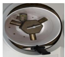
**(b)** Core holders housing 3 cores in the centrifuge machine.
