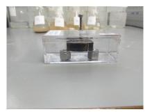
(b) Core aging in test brine at 23°C.
