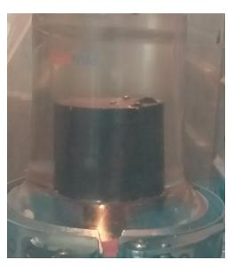
**Figure 6.21:** Segregation due to density difference, seen when changing to brines with lower salinity.
