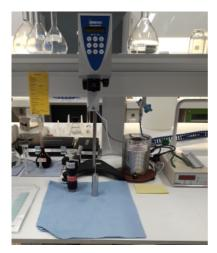
Figure 5.3: Brookfield rotational viscometer.
