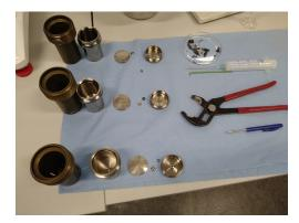
Figure 5.15: Components set-up for the centrifuging process
