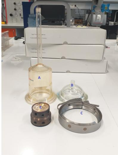
(a) (A) and (B) Upper and lower component of Amott Cell respectively, (C) Metallic core stand and (D) Metal Clutch.
