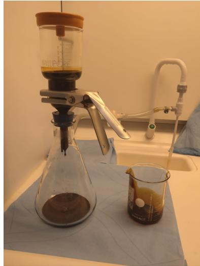
**Figure 5.1:** An image of the oil filtration set-up.
