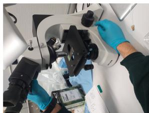
**Figure 5.13:** Checking for asphaltene precipitation, using the microscope.
