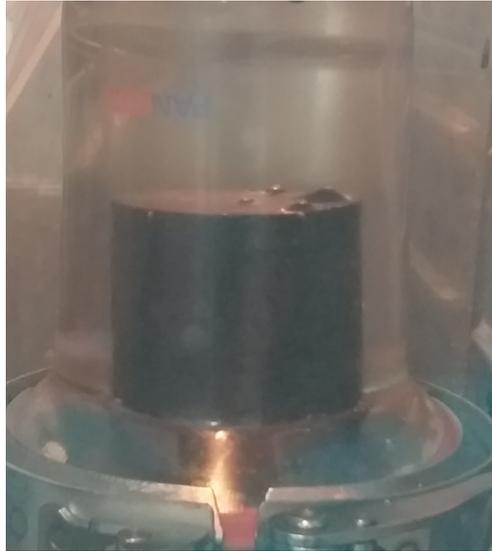
**Figure 6.21:** Segregation due to density difference, seen when changing to brines with lower salinity.
