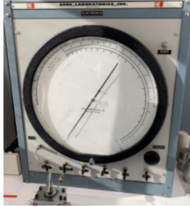
**Figure 5.7:** Helium Porosimeter.
