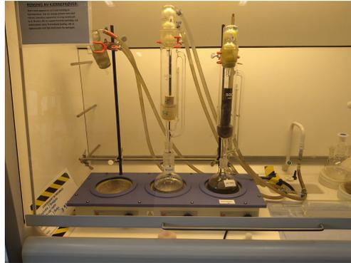
**Figure 5.6:** Core cleaning by Soxhlet extraction.
