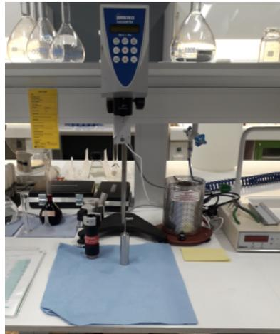
**Figure 5.3:** Brookfield rotational viscometer.
