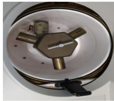
(b) Core holders housing 3 cores in the centrifuge machine.
