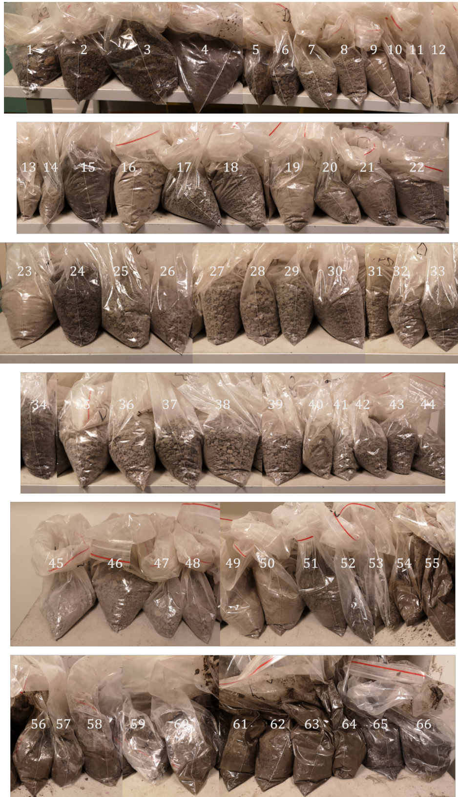
Figure 4.3: Drill cuttings samples collected during drilling with ID nr., with nr. 1 being at the top of the borehole (0-3m depth) and nr. 66 at the bottom of the borehole (195-198m depth). The sampling bags are 5l bags, placed on a table.
