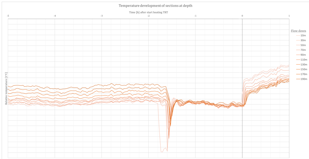
Figure 4.14: Temperature development of the collector fluid prior to and one hour after test start, presented as mean values of 10m sections at depth from optical fiber measurements in the down flow channel of the collector.
