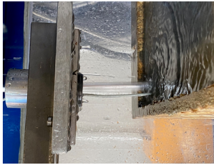
Figure 13.15: Bottom hole assembly with sensor card submerged in water during drilling.
