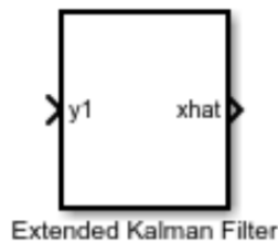
Figure 9.9: Extended Kalman filter block in Simulink with input y_1 and state estimate output \hat{x} .
