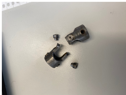
Figure 13.24: Snapped shaft in the universal joint because of to high rotational velocity.
