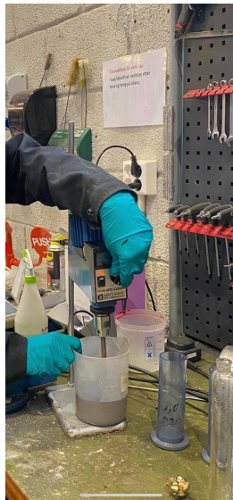
Figure 11.12: Mixing of cement
