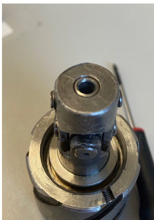
Figure 13.18: Connection between rod and joint made up of two set screws and a steel sleeve.
