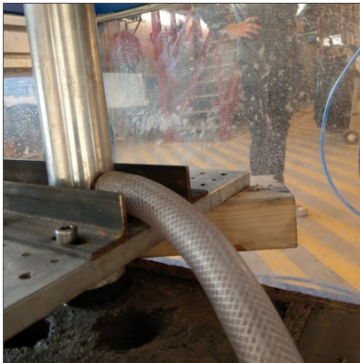
Figure 15.2: Semi-closed loop mud system from 2018 where the interface between rock and riser is sealed to guide flushing up through the rubber hose directly to the drain [52].
