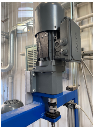
Figure 6.4: Hoisting servo motor.
