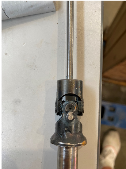
Figure 13.26: Spot welded cap to prevent it from popping out.
