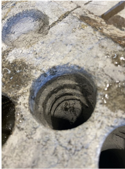
Figure 11.13: Poor hole quality with spiral pattern.
