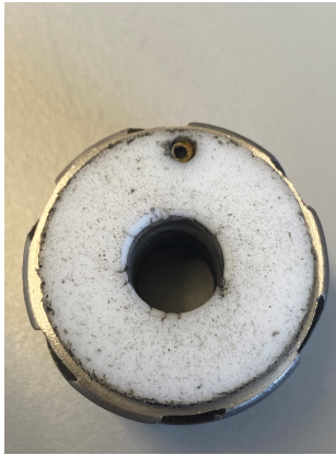
Figure 13.20: Set screw inserted through the packer and into the lower stabilizer to prevent packer from unscrewing.
