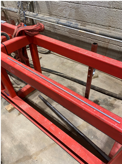
(a) Flat surface used to conduct "rolling test".
