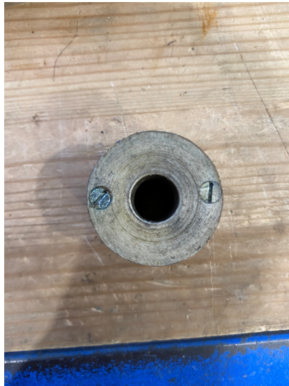
Figure 13.27: Packer made of PEEK with flat head screws to prevent it from unscrewing.
