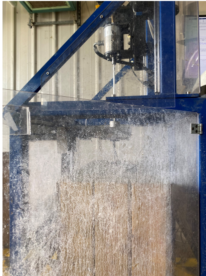
Figure 15.1: Dirty acrylic glass from cuttings squirting when flushed out of rock.
