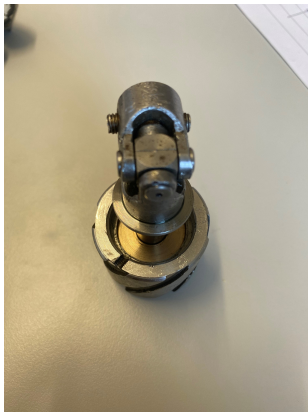
Figure 13.19: Bronze disc in lower stabilizer to minimize friction between joint and inside of stabilizer.
