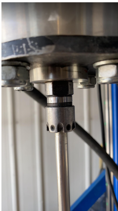
Figure 6.31: Drillpipe connected below the swivel.
