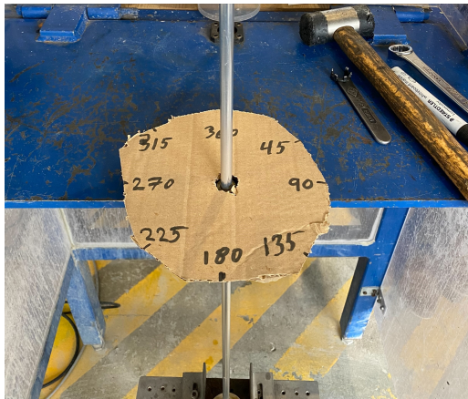
Figure 11.1: Azimuth rotation test setup.
