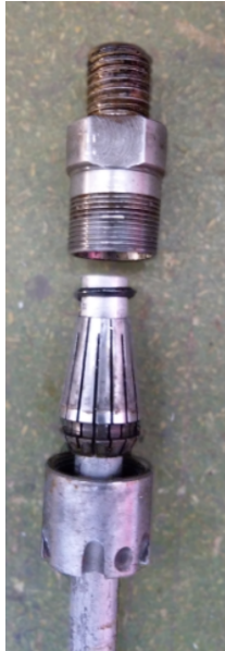
Figure 6.32: From the top: Nipple, spring collet with o-ring, collet nut and drillpipe.
