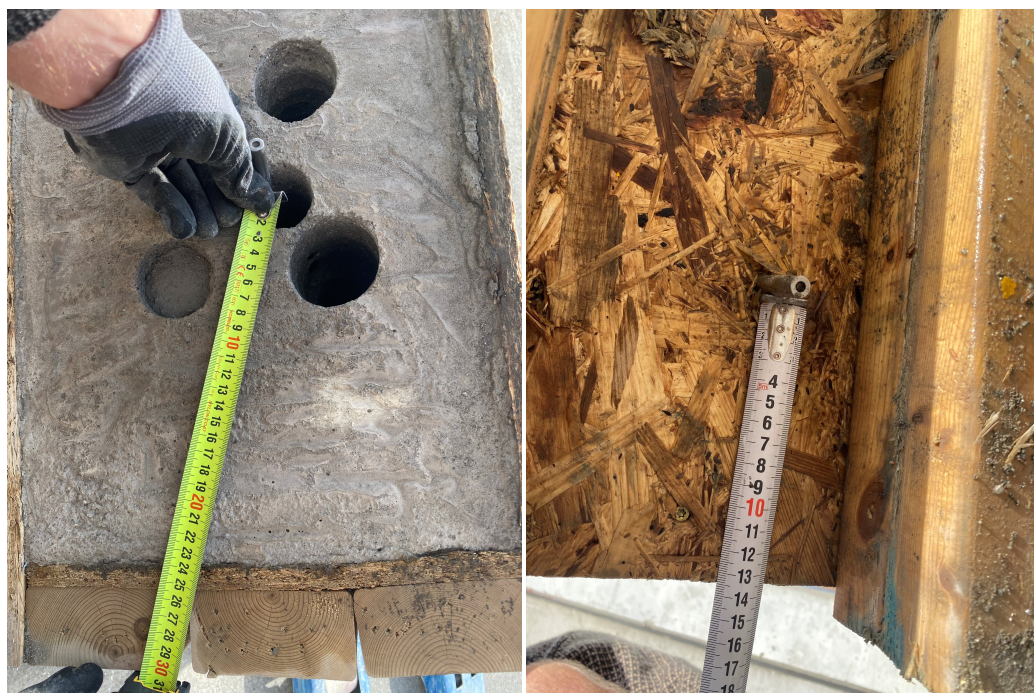
(a) Measured distance from well center equal to 30.5 cm. (b) Measured distance from end point equal to 13.5 cm.
