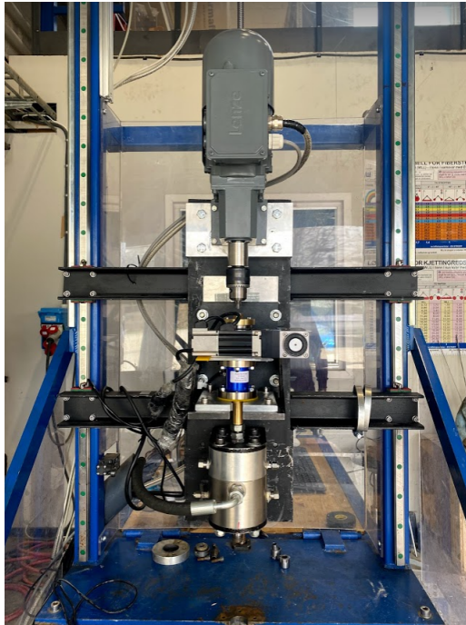
Figure 6.10: Complete rotary system. From top: top drive motor, drill chuck fastener, drill chuck, "T-shaft", azimuth motor, torque sensor, stabilizing plates and hydraulic swivel.
