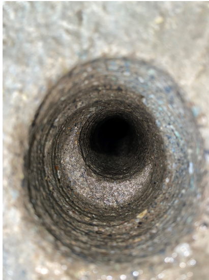
Figure 11.15: Smooth vertical borehole with a clear kick-off point and direction.
