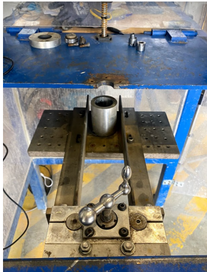
Figure 6.14: Manual hoisting mechanism of the riser.
