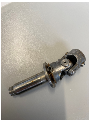
Figure 13.22: Melted steel joint because of friction between the steel disc and the joint.
