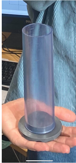
Figure 11.11: Cement test cylinder
