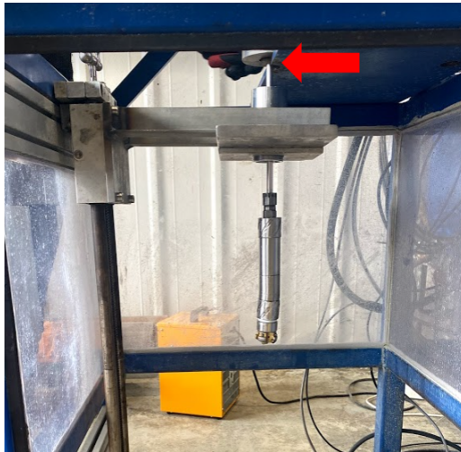
Figure 6.9: Picture of the BHA seen below the derrick floor. Arrow points at upper stabilizer.
