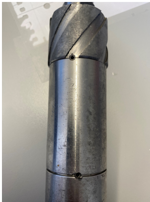
Figure 13.21: Set screws to prevent threads from unscrewing in the joints between components.
