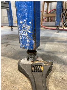
(a) Adjusting rig frame feet.
