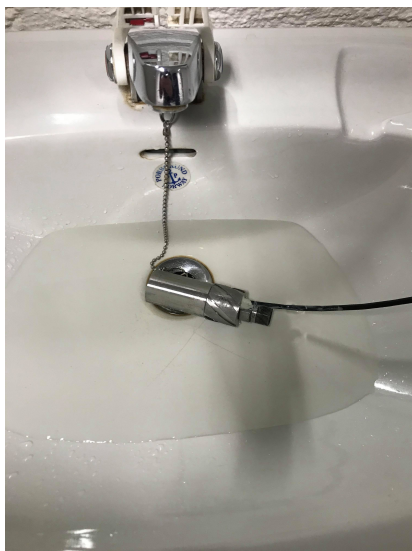
Figure 13.14: Bottom hole assembly with sensor card submerged in water.
