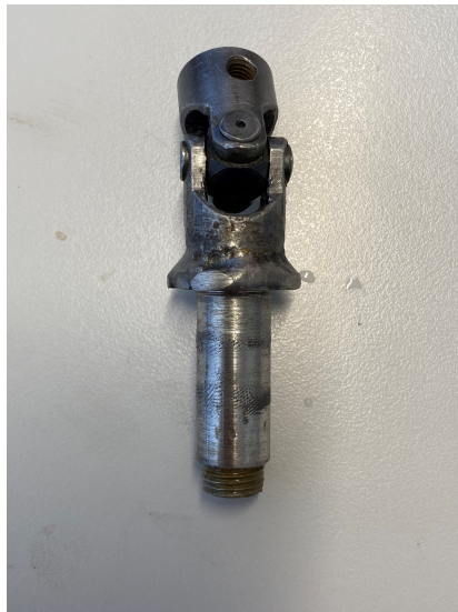
Figure 13.25: Universal joint and drive shaft welded together.
