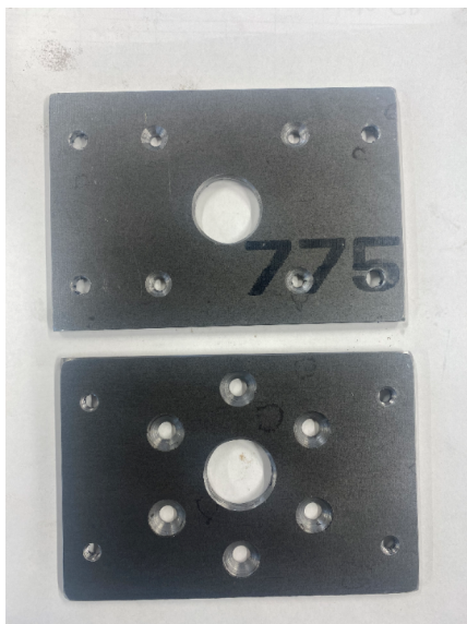
(a) Aluminum plates to mount azimuth gearbox and torque sensor together.
