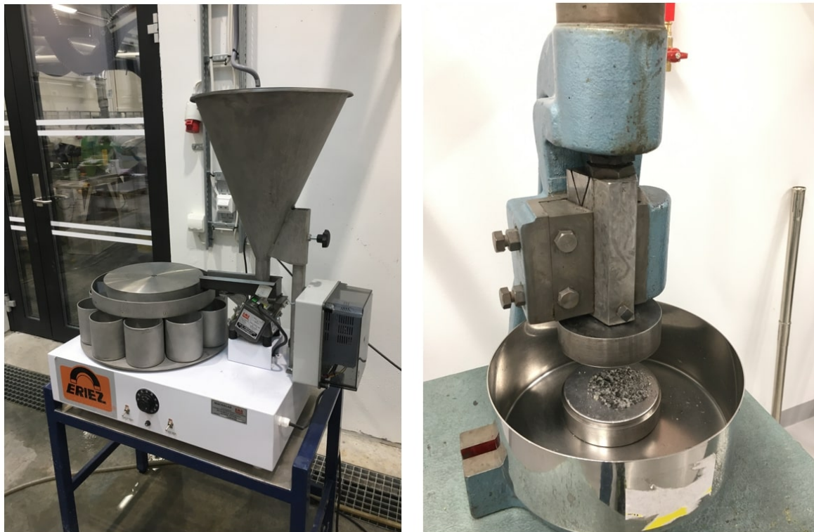
Figure 3.1: Left: Sample separation with the 10-way rotary splitter. Right: Crushing of small samples with the Fly Press Crusher.
