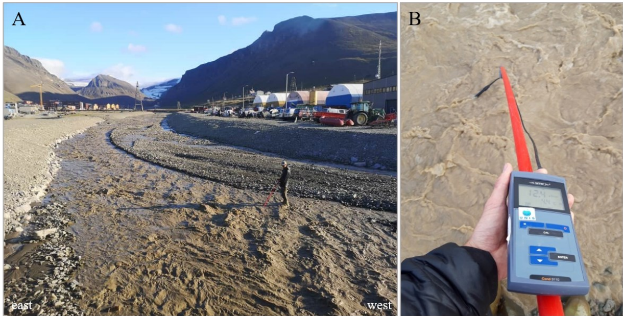
Figure 17: Measuring discharge. A) The writer recording electrical conductivity (EC) in the river after a slug injection of diluted salt. B) To avoid the EC-meter from flapping and catching air in turbulent water, it was attached to a plastic rod and securely submerged.
