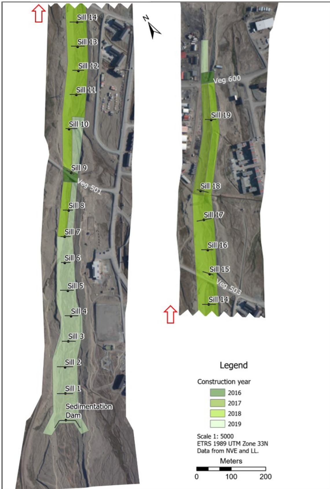
Figure 9: Timeline for construction work (building sills and riprap) in the river by NVE since 2016 and placements of all the sills and the sedimentation dam. Riprap is continuous on both sides from the sedimentation dam to Veg 600.
