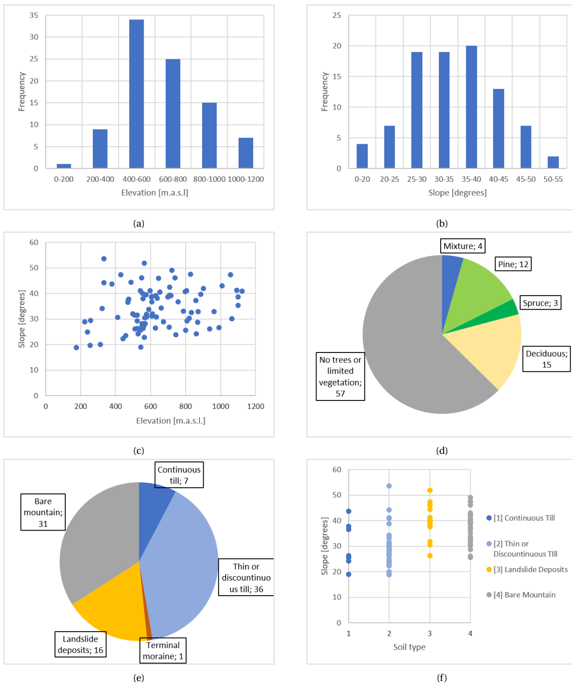
Figure 5.1: Results from the statistical analysis of source areas. Frequencies refer to the number of source area cells , not source areas per se. (a) Elevation distribution. (b) Slope angle distribution. (c) Relationship between slope angles and elevation. (d) Vegetation distribution. "Mixture" refers to varying quantities of pine, spruce and deciduous forest. (e) Soil type distribution. (f) Slope angles for source areas of different soil types.
