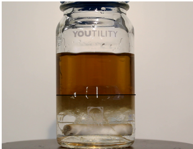
Figure 3.1: Photo of the separation bottle depicting Exxsol™ D60 w/ 300 ppm crude oil, WC 50%. The black line is interface of clean oil, the brown layer between clean oil and transparent water at the bottom is an emulsion layer. Photo taken at T_{in} , time when separation of the phases was completed
