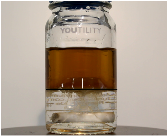
Figure 3.2: Photo of the separation bottle depicting Exxsol™ D60 w/ 300 ppm crude oil, WC 50%. The black line is interface of clean oil and transparent water at the bottom. Photo taken at T_{sep} , time when separation of the phases was completed
