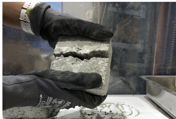
Figure 3.11: Assessing the sample's cohesive strength by hand.
