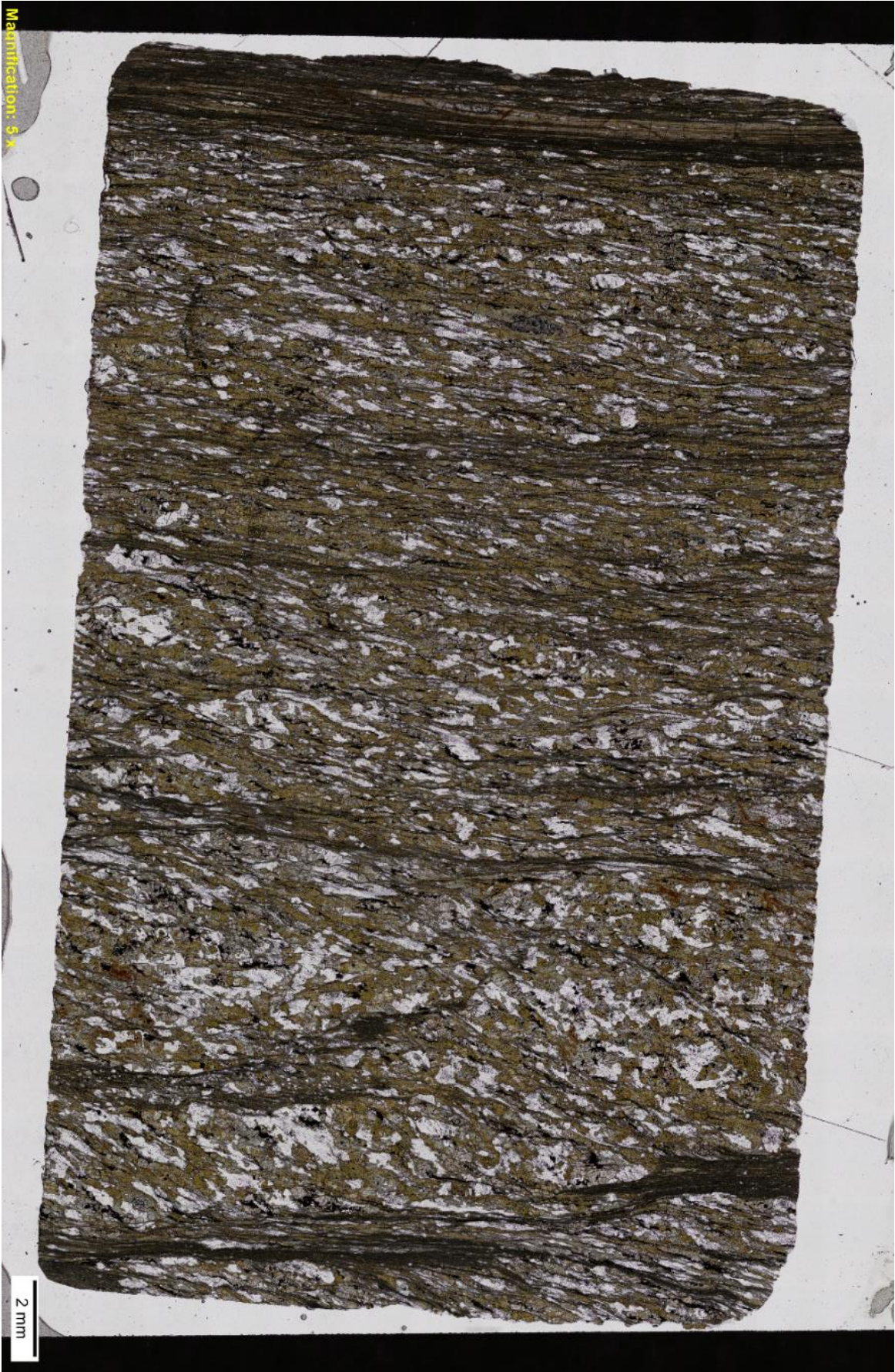
Figure 7.13. Thin section JS15-B in ppl. Deformed hbl gabbro.
