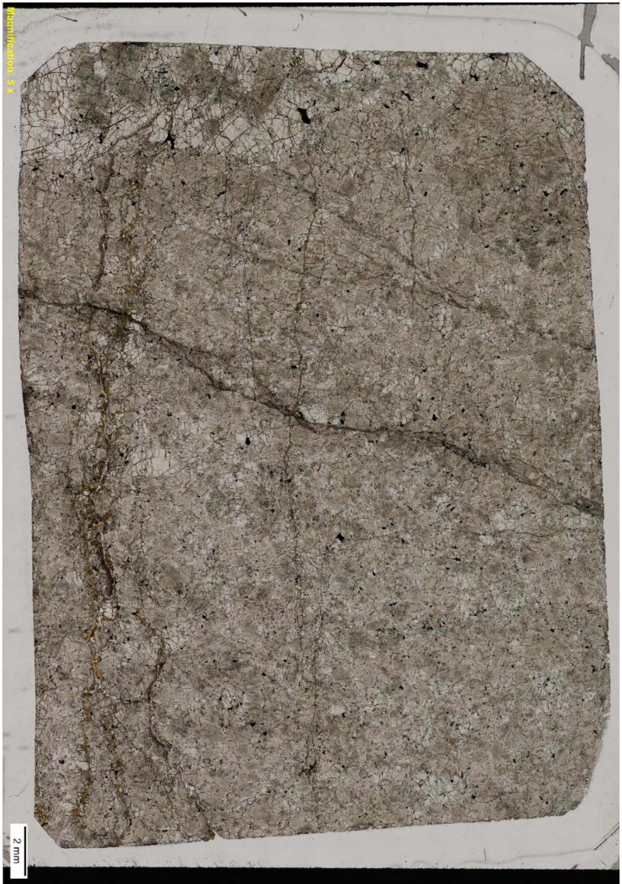
Figure 7.3. Thin section JS_2_10 in ppl. Px rich dyke
