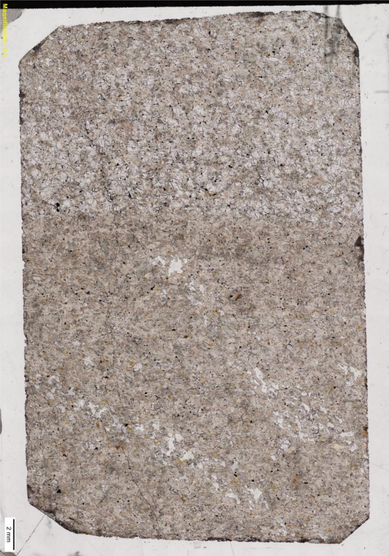
Figure 7.7. Thin section JS_2_18 in ppl. Comp dyke with plag domains
