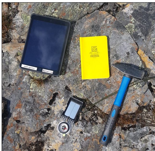
Figure 3.1: Some of the field equipment. Apple iPad, field book, Silva compass, and a geological hammer.
