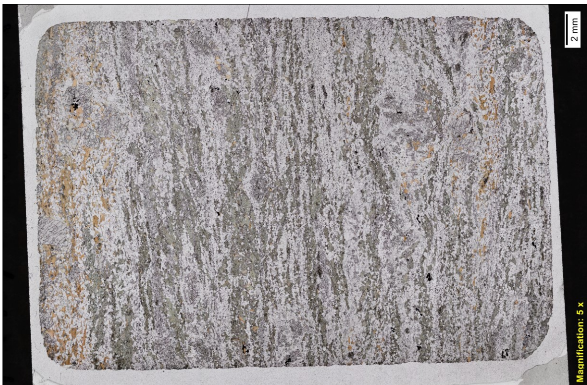
Figure 8.22: Drill core BH4508 at Hellerfjellet. 91.7-91.9 m, 38309. Amphibolite.
