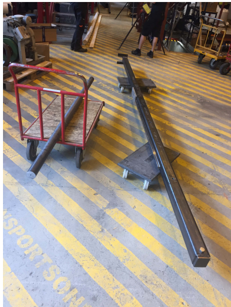
Figure B.11: Drillstring counterweight and supporting structure before assembly.
