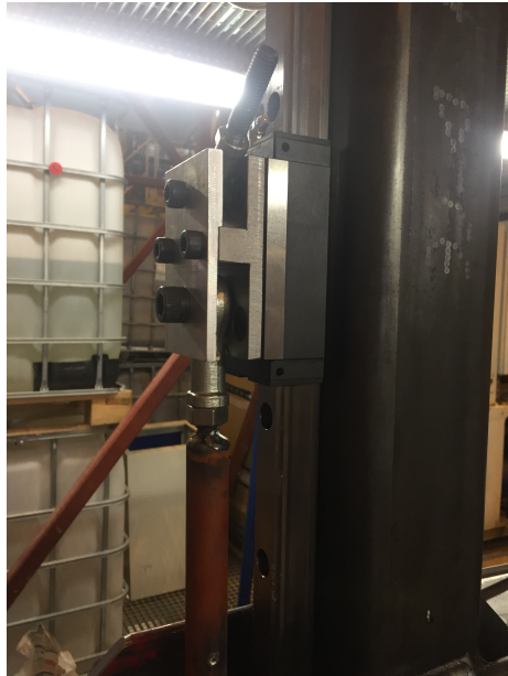
Figure B.18: Slide block mounted to guide rail and drillstring with mount for linear motor
