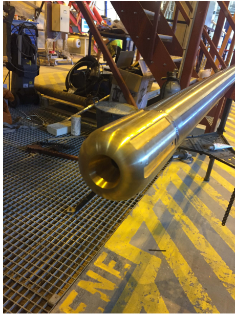
Figure B.6: Brass end piece representing the bit and acting as a funnel guide for the magnetostrictive sensor rod at casing bottom
