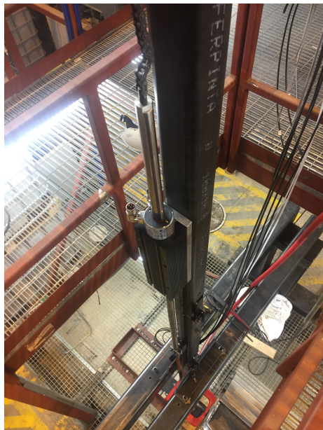
Figure B.19: Linear motor attached to supporting structure attached to sliding block
