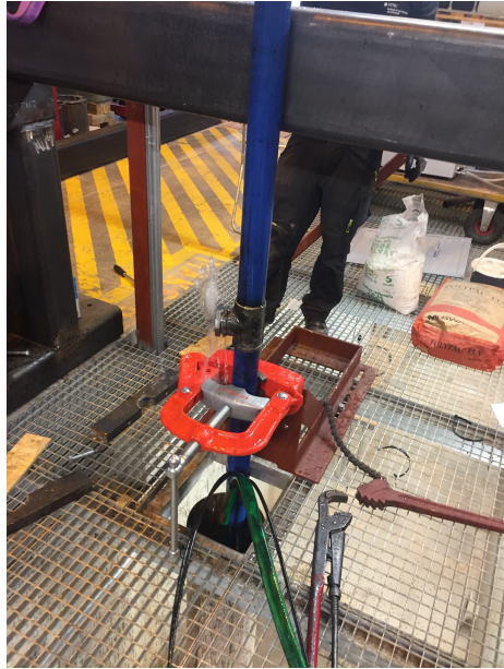
Figure B.4: T-joint pressure sensor mount between casing sections. Here during disassembly with water pushed out by the hydrostatic column of remaining water within the casing above the T-joint
