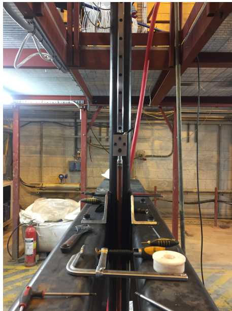
Figure B.17: Supporting structure mounted with guide rail and drillstring attached to slide block
