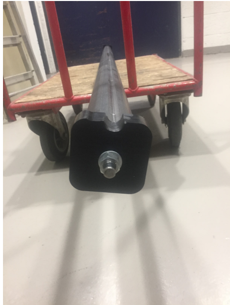
Figure B.12: Counterweight with plastic guides for sliding within the supporting structure. Counterweight and guide grooved out to account for a weld within the supporting structure.
