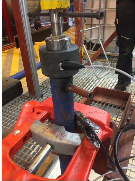
Figure B.2: Casing Mounted in Slips with PVC Sleeve for Temperature Sensor Mount and Steel Spacer below to Avoid Any Damage to the Sensor Fitting
