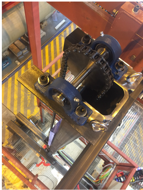
Figure B.22: Steel cogwheel with bearings for chain connecting linear motor and counterweight
