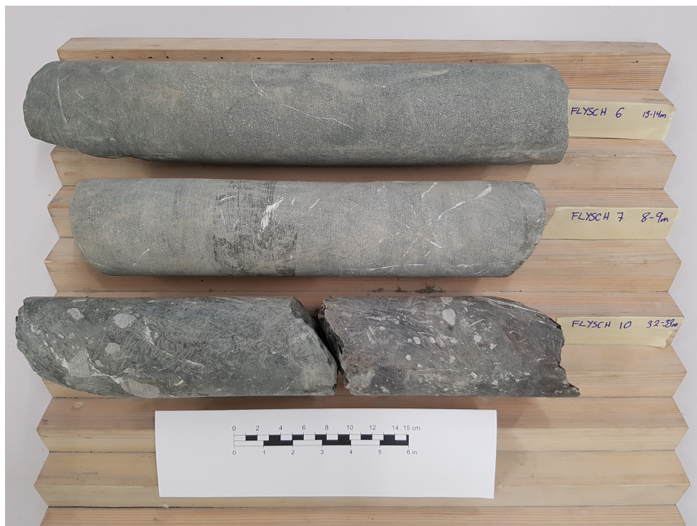
Figure 5.2. Flysch cores from Moglice headrace tunnel. F6 and F7 are sandstone flysch, while F10 is a clay flysch.
