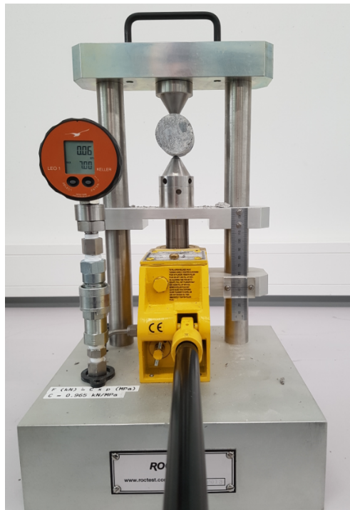
Figure 5.3. The setup of the point load strength test for diametral testing on a rock core.
