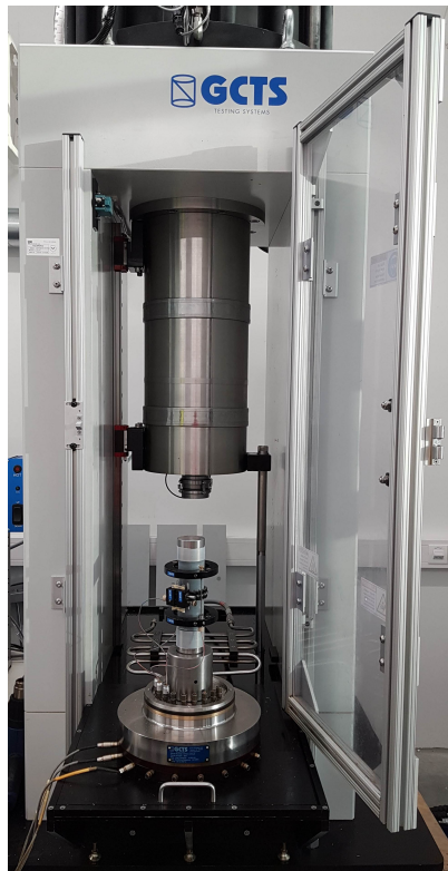
(a) Photo after Aasteboel (2019) of the apparatus used to test uniaxial compressive strength.
