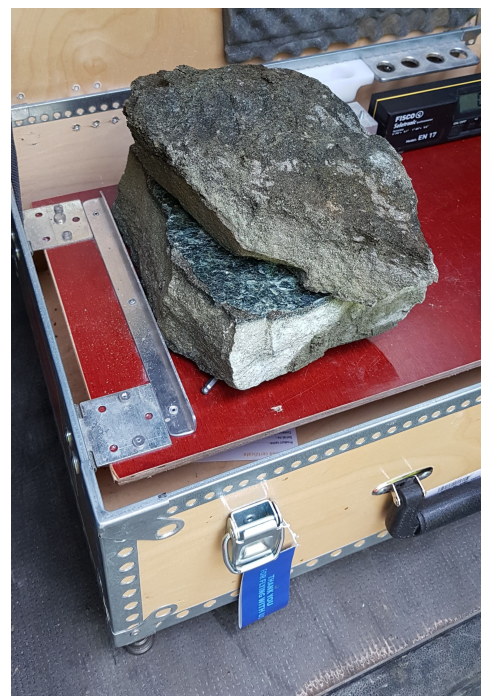
(b) Photo from Aasteboel (2019) of a pair of blocks to be tested on the tilting platform.
