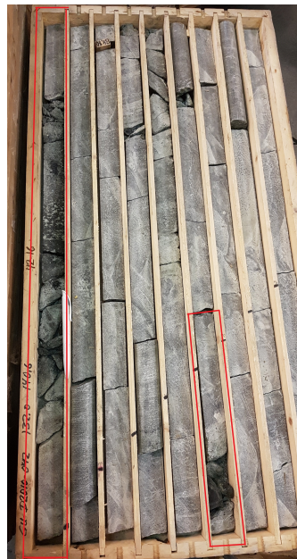
(e) Photo of the rest of the widest eclogite and amphibolite zone and another eclogite zone in drill core GU-2010-042.
