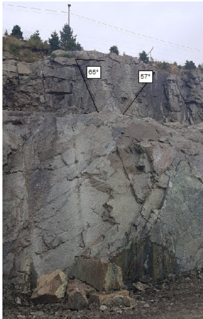
(a) Photo used to measure the dip of the western and eastern joints defining wedge 3.
