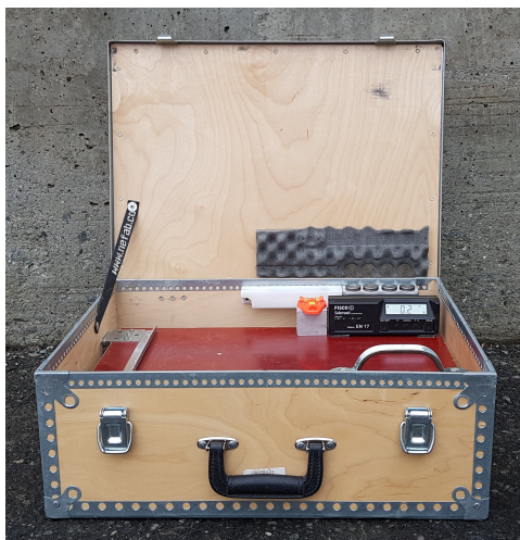
(a) Photo from Aasteboel (2019) of the tilting platform used for tilt testing.
