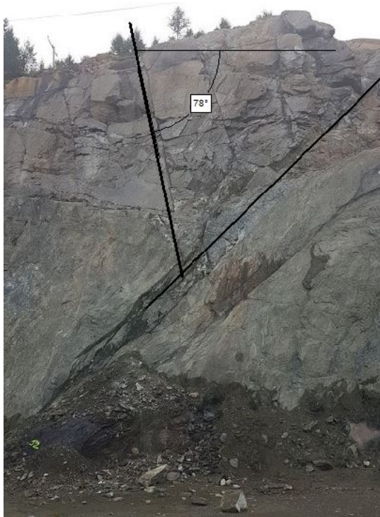
(a) Figure of the photo used to measure the dip of the western joint defining wedge 1. The value of the measured dip is indicated.
