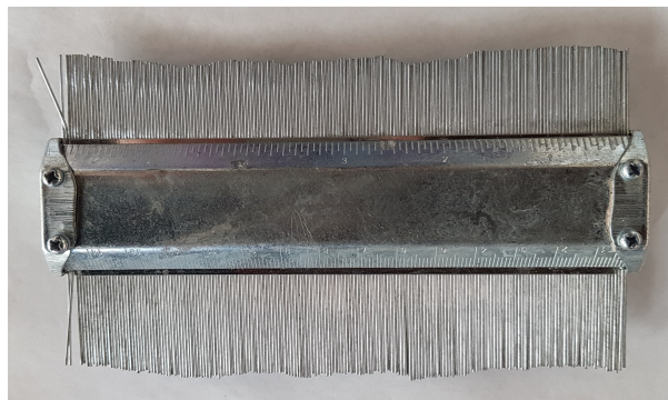
(a) Photo after Aasteboel (2019) of the steel profile gauge used to take imprint of surface roughness of joint walls.
