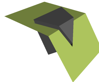
(b) Figure of the wedge formed when the tension crack is defined by the foliation located at the innermost part of the bench.
