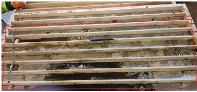
(e) Photo of contact zone in drill core GU-D2010-041.
