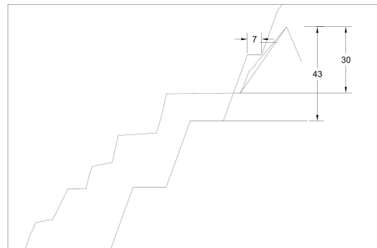
(b) Geometry of the current slope and the slope defined in the life of mine model, by wedge 1.
