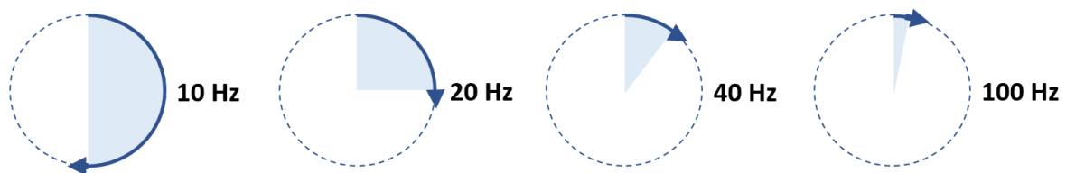
Caption: Measuring drill string rotation at different sample rates.
