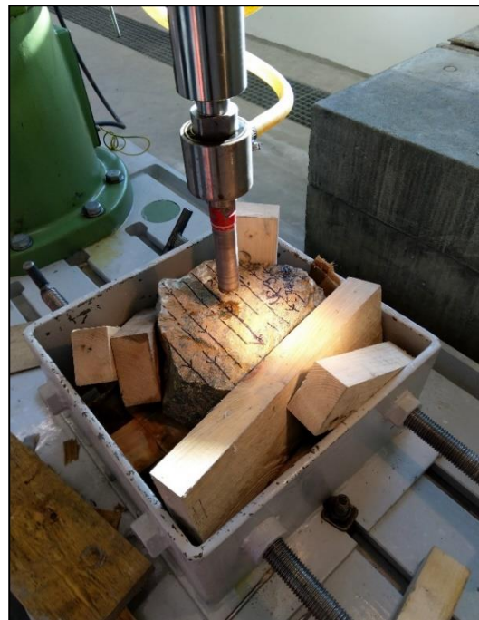
Figure 3-2: Drilling cylinders on the marked surface.
