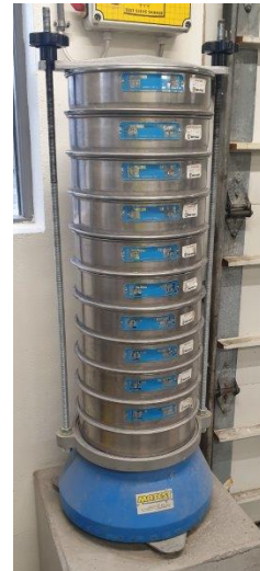
Figure 4.2: Laboratory test shaker with a sieving column.
