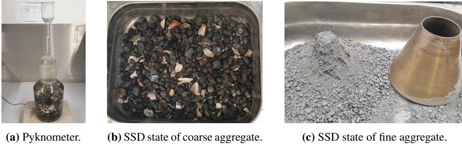
Figure 4.3: Particle density and water absorption test procedure.
