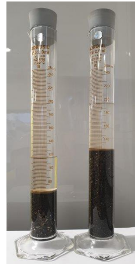
Figure 4.8: Determination of presence of humus and fine mud and clay content.
