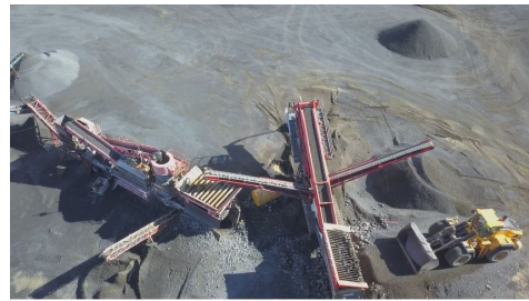
(b) Primary crushing with a cone crusher, screen and stockpiles.
