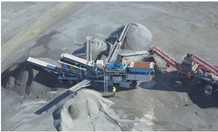
(a) Secondary crushing with a VSI crusher, screen and stockpiles.
