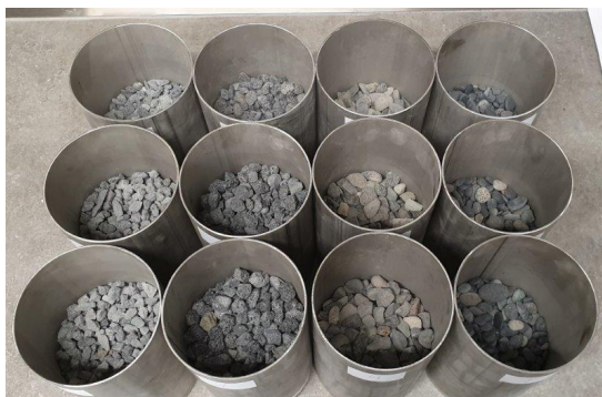
(a) Coarse aggregate test specimens in cans prior to soaking.
