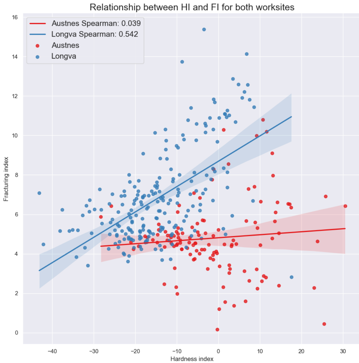
Figure 7.14: Scatter plot of int. hardness and fracturing grouped by the two worksites. Linear association incl. Spearman correlation coefficients between the respective groupings are annotated.
