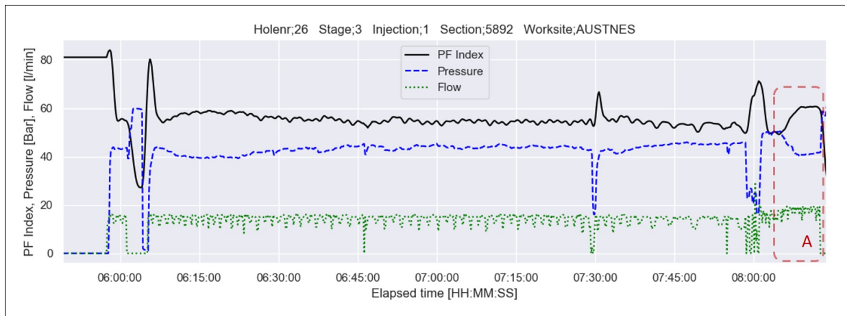
Figure 7.4: Grout pressure, flow and calculated PF index with time for three boreholes from the Austnes Worksite, ch. 5892. These are some examples where indications of HJ events were found, marked by red boxes.
