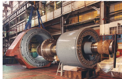
(b) Induction motor for ship propulsion (Kirtley et al. 2015)
