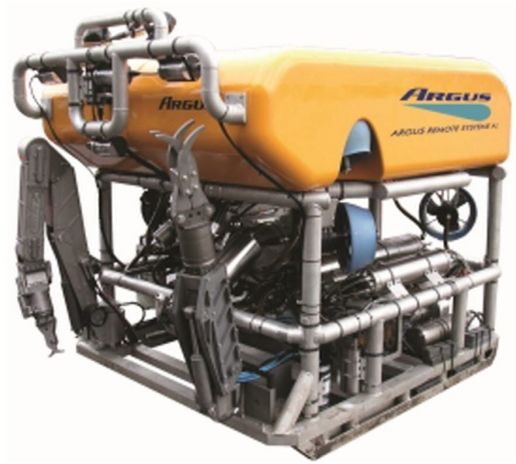
(b) Prototype of ROV for net repairs (Sintef.no)
