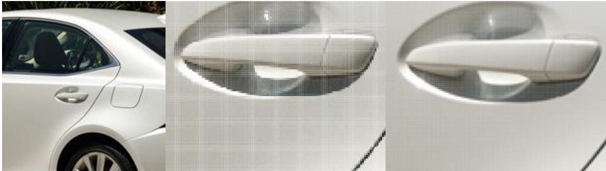
Fig 2.15: Shows how a car image (to the left) is impacted by being resized by nearest neighbour (in the middle) and bilinear interpolation (to the right). Here the compressed images are magnified 930%. Tabora [50]
