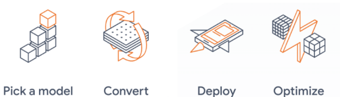
Figure 2.6: The flow of operation using TensorFlow Lite. Taken from [Ten, 2020a].
