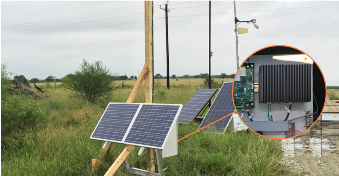
Figure 1.2: An example of solar panels being used to provide sustainable energy for a deployed IoT device. Taken from [OnL, 2017].
