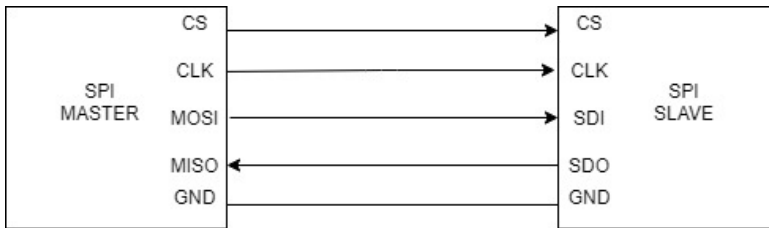
Figure 2.2: SPI communication. Data is transmitted between master and slave entities.
