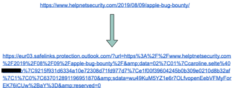
Figure 4.5: Example of the change in presentation of URLs with the new email security solution in the case organization.
